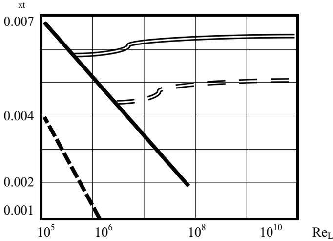
Fig. 1. Example of a change in the friction drag coefficient as a function of the Reynolds number for a flat plate  $\{c_{xt} = f(Re_L)\}$  in different types of flow, including the impact of roughness. Laminar flow: dotted line. Turbulent flow: continuous line. The impact of the same absolute roughness in turbulent flow: double lines (continuous for a shorter plate and dotted for a longer plate)
