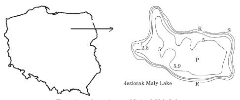
Fig. 1. A morphometric map of Jeziorak Mały Lake: S – sites with pipes from separators which drain stormwater, K – sites with stone accumulation created in 1997, R – sites with macrophytes, P – pelagic zone
