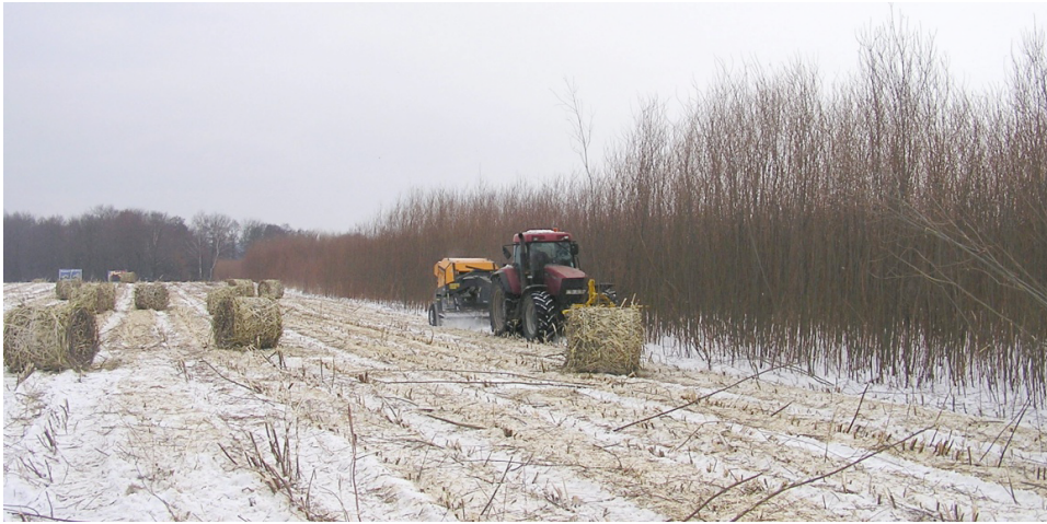
Fig. 1. A set for willow harvesting, consisting of Biobaler WB 55 and a Case IH MX170 tractor
