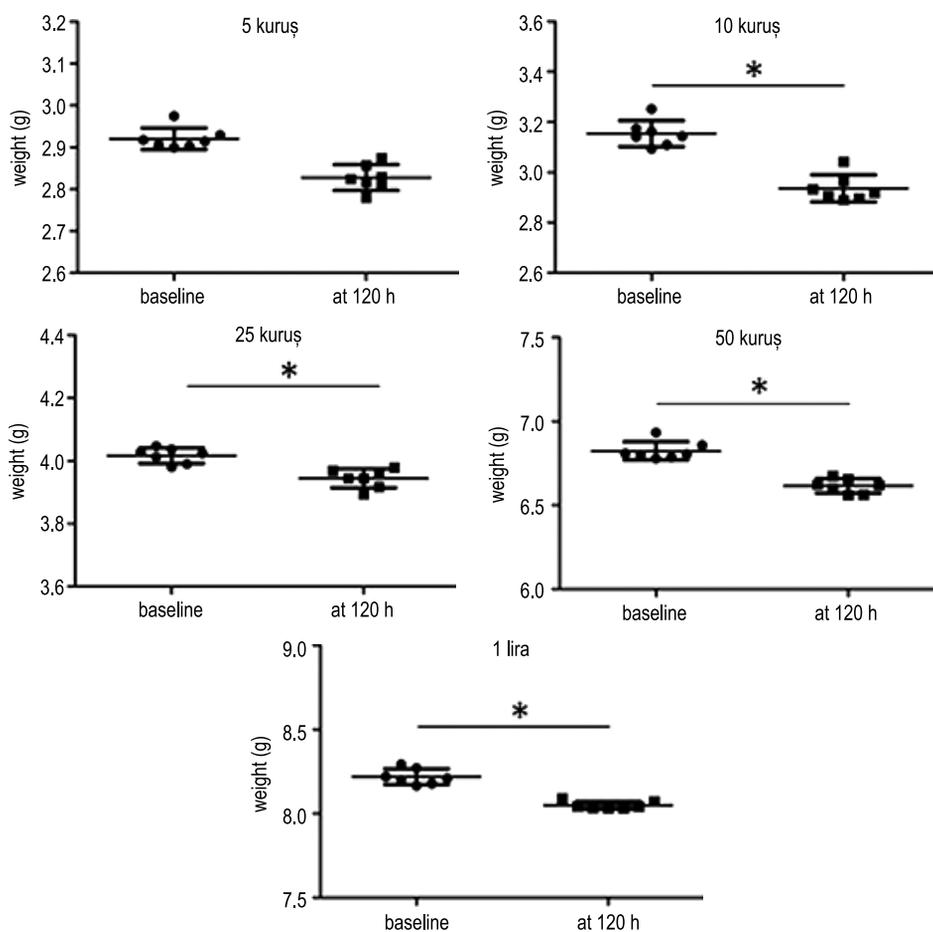
Fig. 1. Weight loss of Turkish coins before and after 120 h exposure in simulated gastric juice
