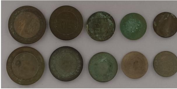
Fig. 2. Progressive corrosion of Turkish coins after 120 h in simulated gastric juice
