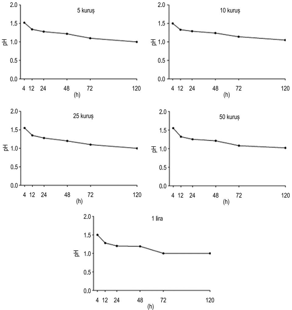
Fig. 3. pH values of simulated gastric juice with immersed Turkish coins during 120 h
