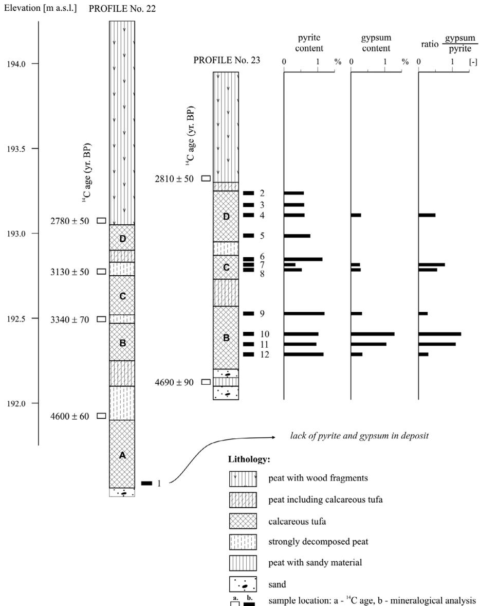
Fig. 2. Mineral composition of the calcareous tufa, and  $^{14}\text{C}$  age of the peats
