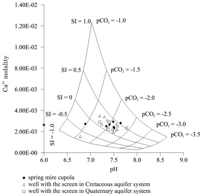
Fig. 5. Groundwater pH vs.  $\text{Ca}^{2+}$  concentration with theoretical equilibrium curves of calcite saturation index and partial  $\text{CO}_2$  pressure (PHREEQC calculation results)
