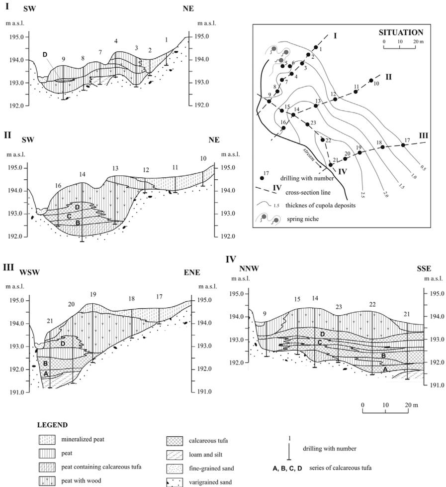
Fig. 3. Geological cross-sections through the cupola
