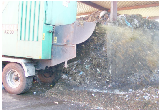
Fig. 2. Shredding of the organic waste (KLIMAS 2014)
